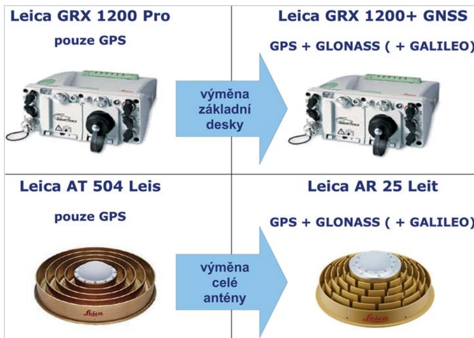
Obr. 6 Princip uprade stanic CZEPOS v letech 2011 a 2012
