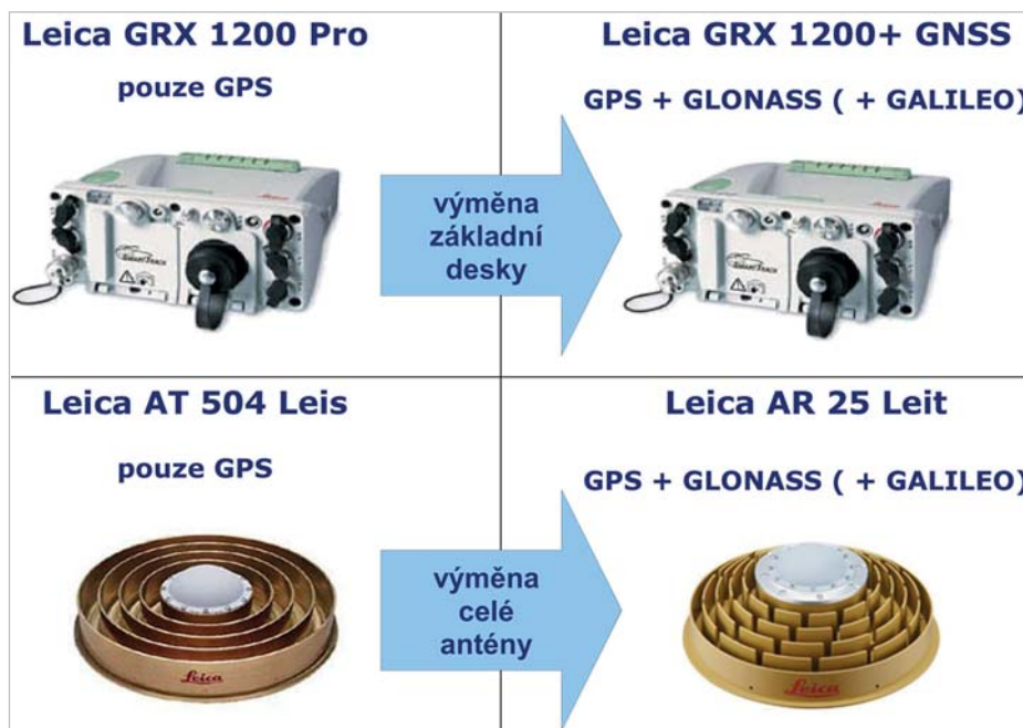
Obr. 6 Princip upgrade stanic CZEPOS v letech 2011 a 2012
