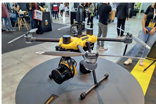
Obr. 7 Dron Argosdyne s LiDAR-om YellowScan (foto: P. Michalovič)
