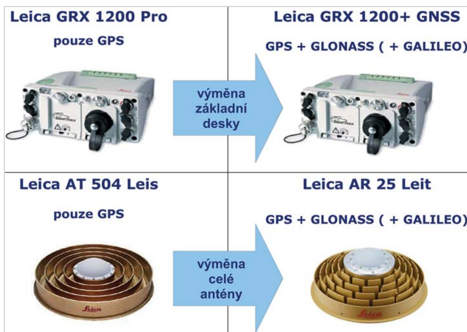
Obr. 6 Princip upgrade stanic CZEPOS v letech 2011 a 2012
